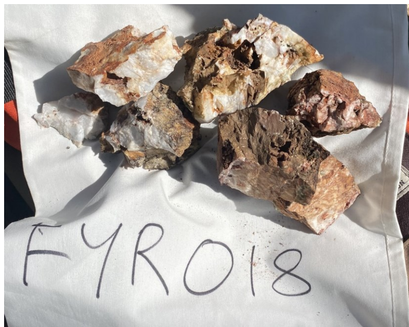
Photos 3 and 4 Forsayth Iron (Fe) and Manganese (Mn) ridge. Photo Left: 5.4g/t Au 0.365% Mn 0.45% Pb 0.12% Cu. Photo Right: Mineralised vein quartz 25.6g/t Au and 16.3 ppm Ag
