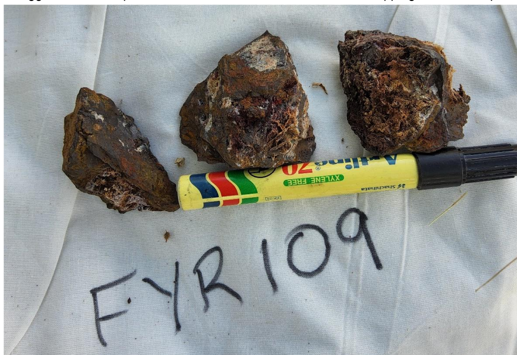
Figure 7. Gossanous vein quartz. Sample FYR 109 (16.15 g/t Au & 28.3 g/t Ag)
