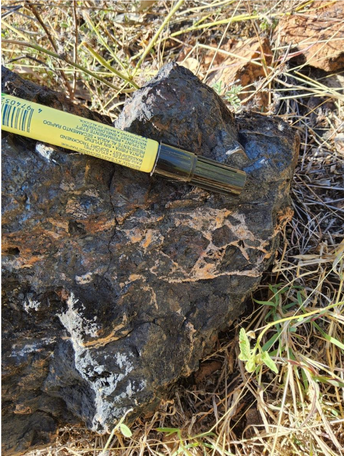
Figure 8 Brecciated ironstone with quartz matrix
