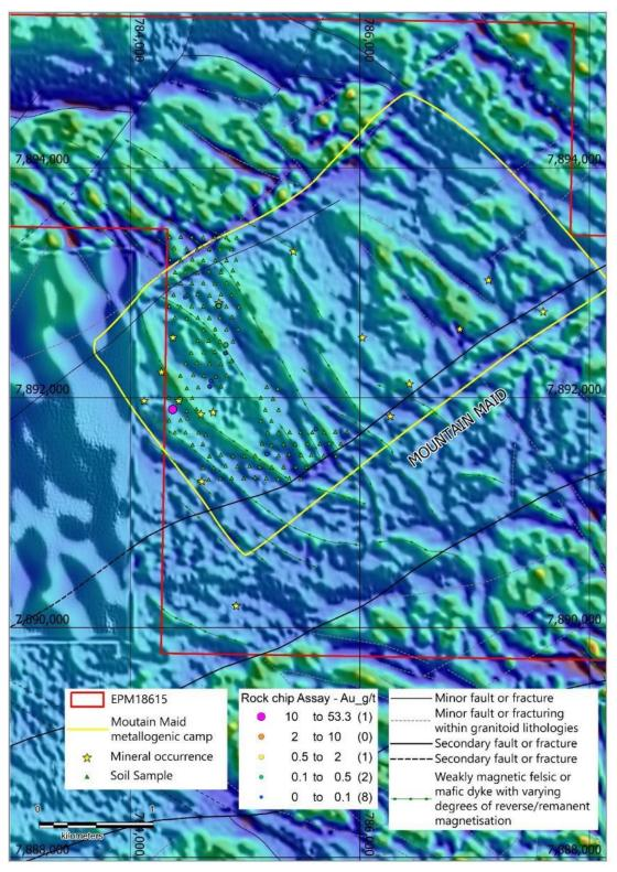
Figure 10 – Dividend Gully Prospect rock chip Au assays and soil samples on Magnetics RTP 1vd.
