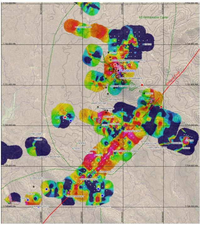
Figure 19 Mt Remarkable Camp Soil Gold Grid Au ppb (white dots are soil samples this reporting period) along with 2022 stream sediment (blue stars) rock chip (red stars) samples and drill hole PLJVDD001.
