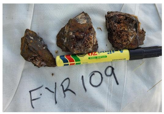
Figure 4 Gossanous vein quartz. Sample FYR 109 (16.15 g/t Au & 28.3 g/t Ag).
