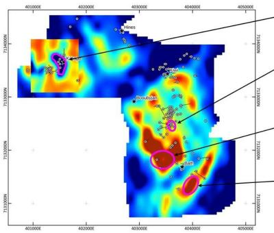
Booubyjan - Depth slice at 175m through the 3D Inverted Chargeability Kakapo - Depth slice at 175m through the 3D Inverted Resistivity
