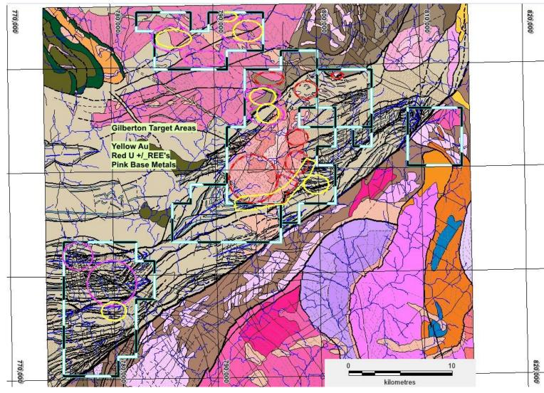
Figure 5. Boad target areas for Gold, Base Metals, Uranuim+/- REE's.
