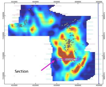
Figure 10 Section through hole ABJ004. Shells are 3D inverted chargeability (15.0 to 30.0 mV/V). Drill trace coloured by S (Sulphur).
