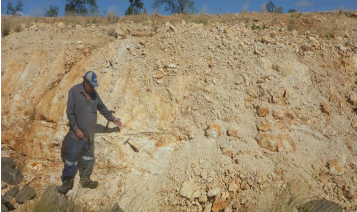
Figure 5. REE Target - Kaolinitic sediments of the Walumbilla Formation exposed as a scarp.
