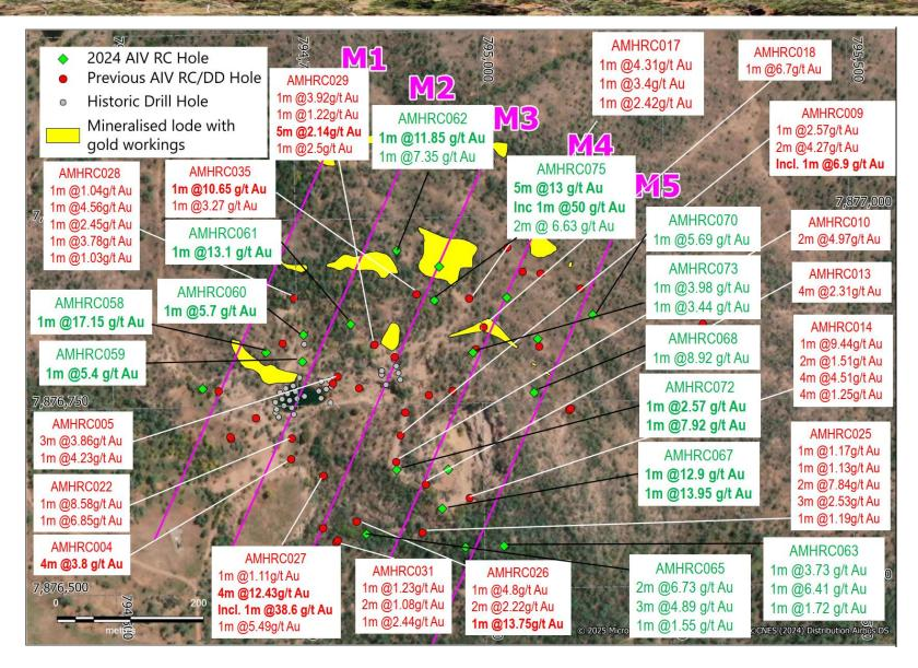
Figure 3 Mt Hogan Drilling Plan View.
