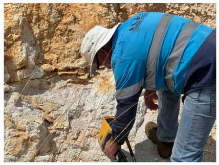
Figure 5. REE Target - pXRF sampling of white weathered kaolinitic fine-grained sediments adjacent to the prominent scarp as shown in Figure 4
